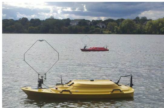
Fig. 1. The robotic systems used in field experiments. The 2-meter long boats were designed to track invasive fish autonomously. Each one is equipped with wireless communications, directional antenna used as bearing sensors, a navigation suite, and computing hardware. Our algorithm was implemented on this system and was shown to localize targets with small uncertainty.
