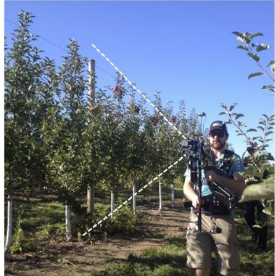
(b) The sensor suite mounted on a hand-carried steadicam, providing side view of plants (towards the left in this image, pointing at a row of apple trees). The white dashed lines show the vertical field of view of the system. This arrangement provides rich data on fruits, canopy, and trunks. Such data can also be acquired with the sensor suite mounted on a UAV flying between trees.
