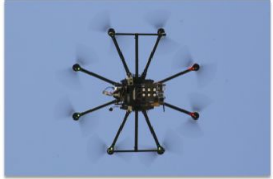
(a) The sensor suite mounted on a UAV, scanning plant canopies from the top with the sensors pointing downwards.
